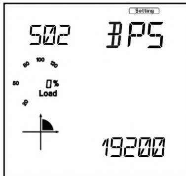
Figure 6-3 System Parameter Setting - S02 Baud Rate
