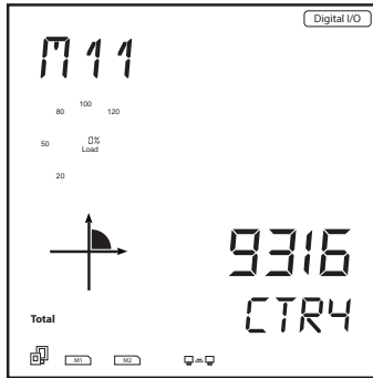
Figure 5-24 Digital Input Pulse Count from Meter's Display
