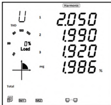
Figure 3-25 Harmonic Distortion Reading
